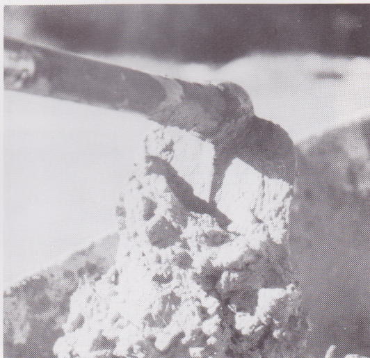
Fig. 5.1 – The soil in (a) is too dry for adobe construction and the soil in (b) is at the correct moisture content
