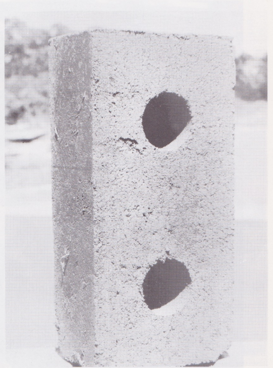
Fig. 6.9 – A Cinva-ram block cast with holes for cyclone bolts or vertical reinforcement
