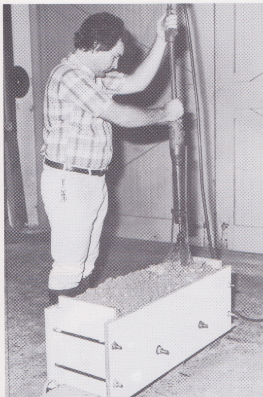
(b) A rammed-earth test specimen being compacted
