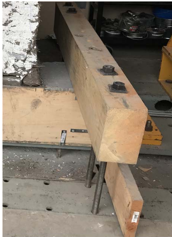
Figure 9: Wall Testing Restraint System.
