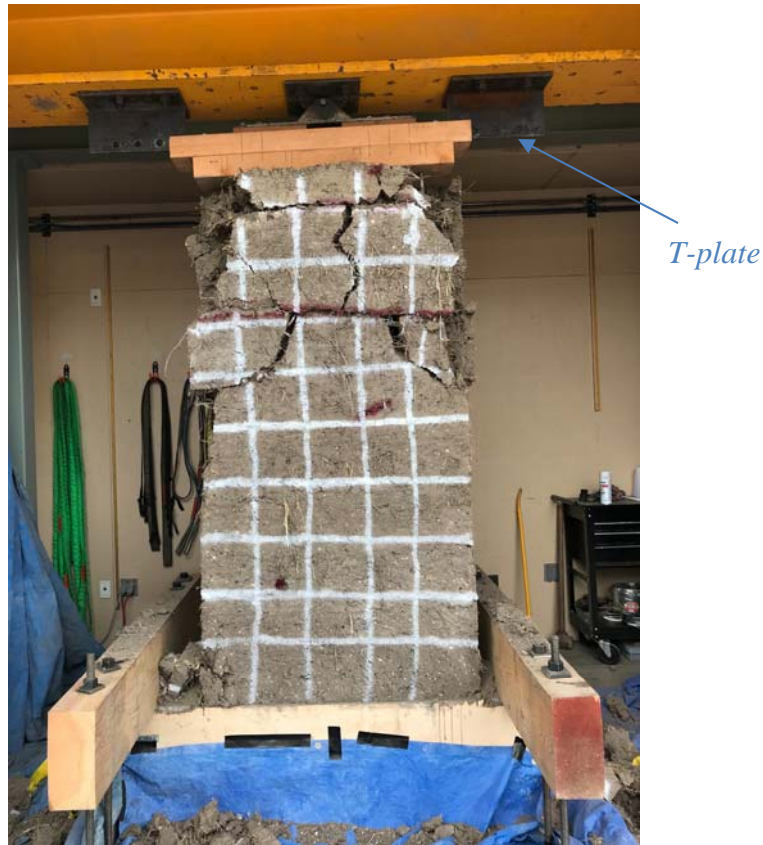
Figure 14: Wall 3 (Medium Reinforcement) After Testing.
