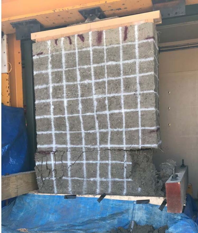
Figure 16: Wall 4 (Light Reinforcement) After Testing.
