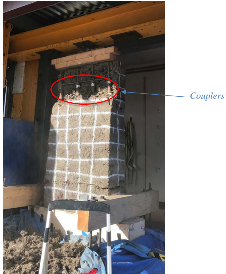
Figure 12: Wall 2 (Heavily Reinforcement) After Testing.
