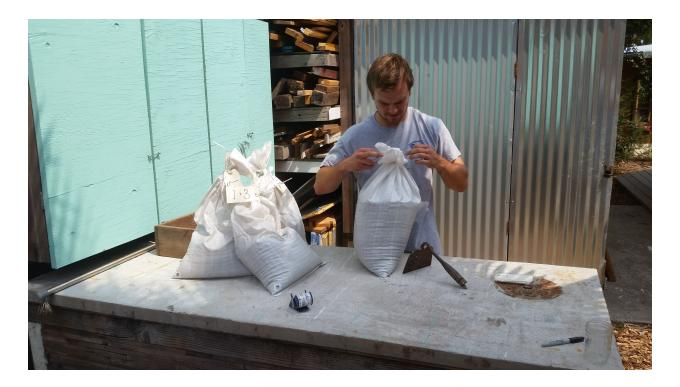
Bagging the mix samples, to take to SCU to make the cob Test Blocks. These will be 12" cubes for compression and 6"x12"x36" beam block for rupture.
